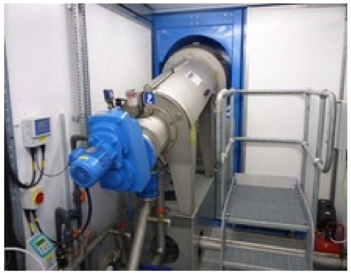
The feed sludge during the trial varied from 4.6 to 5.15% DS with an average active polymer usage of 4.7-4.8 kg/tDS with an average cake dryness of 33% and minimum of 28.6%.
