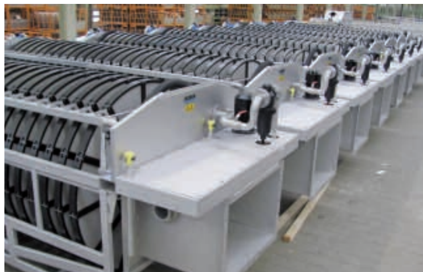
8 RoDisc® 24 screens in the factory just before delivery with the clearly visible discs consisting of individual plastic segments
