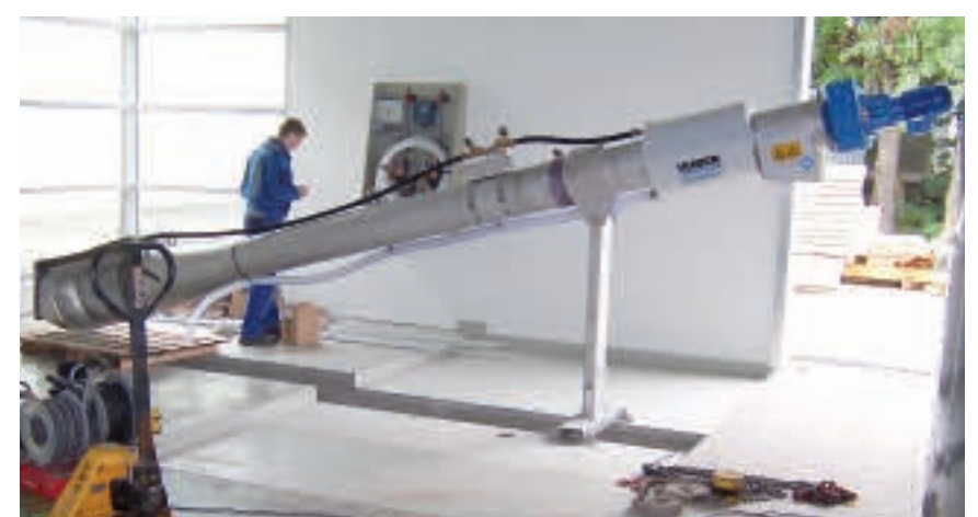
HUBER ROTAMAT® Micro Strainer for separation, washout and compaction of solids from the combined water generated in the company's production process
