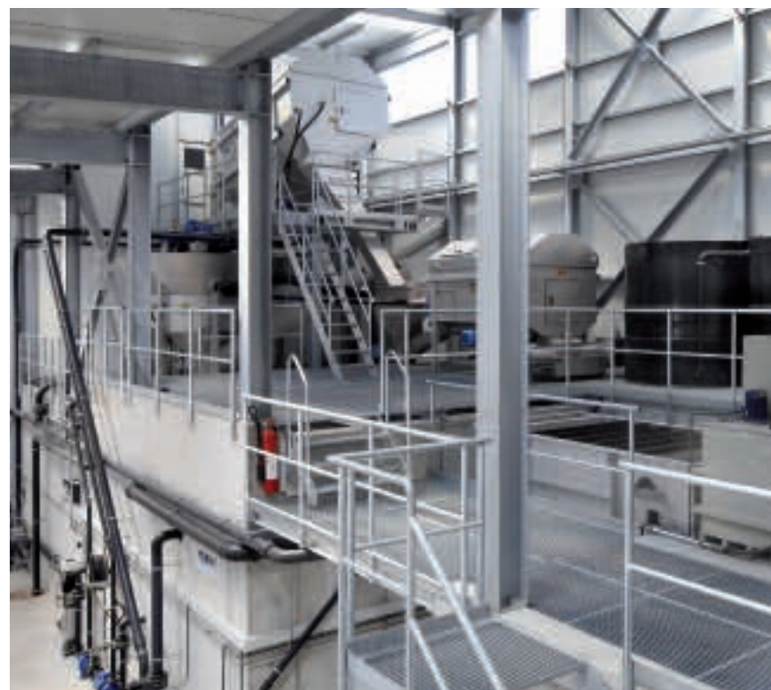
Grit treatment: HUBER Wash Drum RoSF 9 with two subsequent HUBER Grit Washer RoSF 4 units, coarse material washer, ROTAMAT® Rotary Mesh Screen RoMesh® for organics removal and compaction
