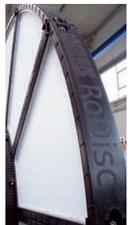
Plastic segments of a HUBER RoDisc® screen
