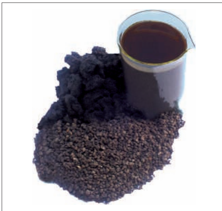
Typical sewage sludges: liquid – pasty – solid
