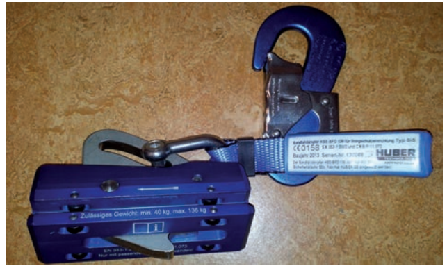
SIS 2/3 Fall arrestor type S5b with safety traveller, approved for a weight of 136 kg
